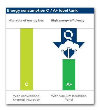
A 300 litre tank with the efficiency label C has, e.g., a power loss of approx. 85 W, while the same tank with an A+ label has a power loss of less than 36 W. That is more than 50% less or a saving of more than 1 kWh per day.
